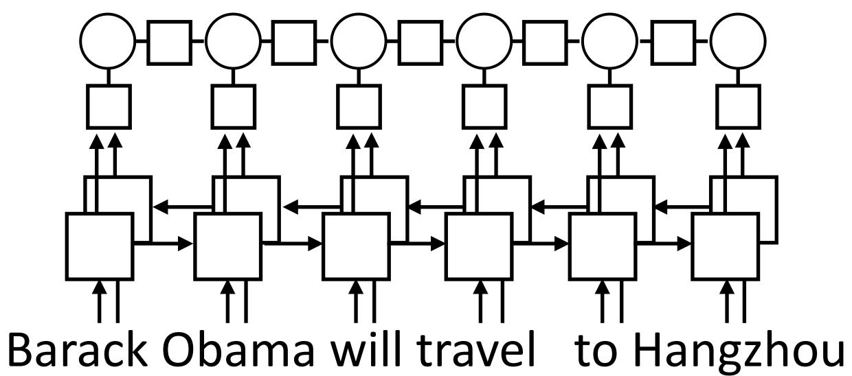
Neural CRFs: bidirectional LSTMs (or some NN) compute emission potentials, capture structural constraints in transition potentials
